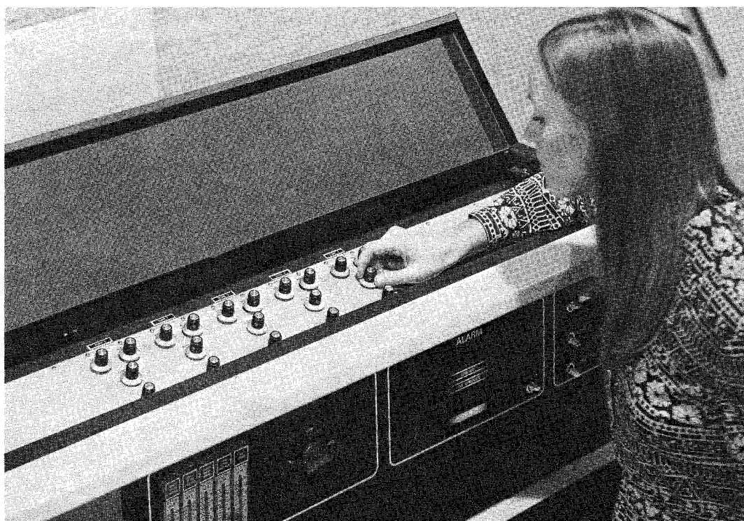
Blind controls such as zone trimming are located under a hinged panel where access is convenient but out of the way of idle fingers.
